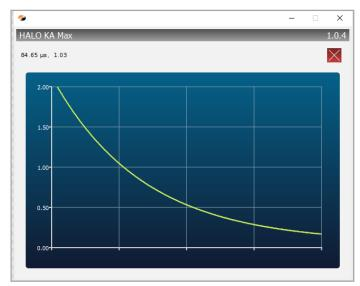
Ring-down data is streamed live to your computer to check the analyzer status remotely and in real-time.
